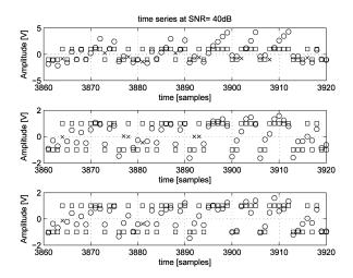
Fig. 4. Time series of distorted data symbols (top), data symbols after the linear equalizer (middle), and data symbols after nonlinear equalizer (bottom). " $\Box$ " denotes the originally transmitted symbol, " $\circ$ " denotes correctly detected symbol for each equalizer, and "×" denotes incorrectly detected data symbol for each equalizer, respectively.
