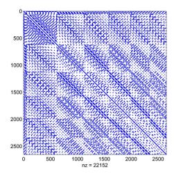
Fig. 5. Autocorrelation matrix of the data vector  $\mathbf{r}[k]$ . The matrix has 2652 × 2652 elements, where 22 152 are nonzero which reduces computational complexity because of the sparsity.
